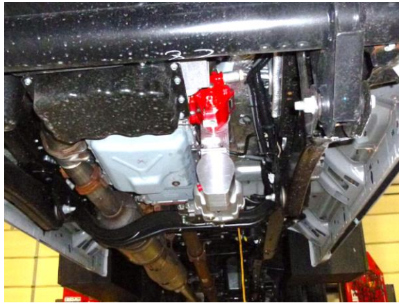
Bolt the hydraulic pump to the "HYDRA DRIVE"*
